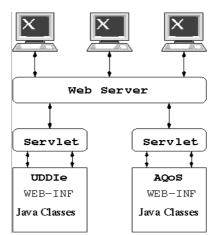
Figure 7: When using UDDIe, a client sends a request as an XML message to the Servlet, which parses the request, and forwards it to the registry
