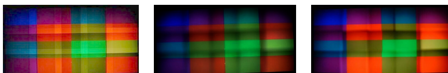
Fig. 13. The fifteen projector tiled display before blending (left), after software blending (middle), and after optical blending using physical mask (right).
