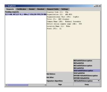
Fig. 7. SimplerCA interface for approving certificate requests
