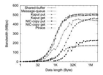
Figure 4: Comparing the performance of the data transfer mechanisms.
