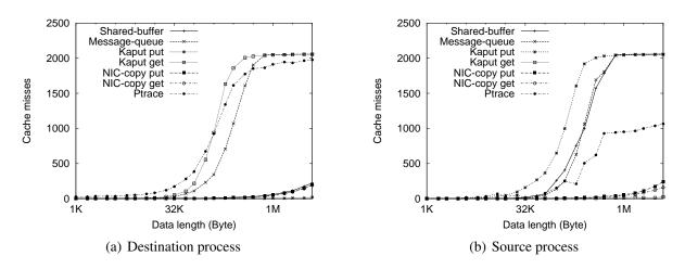
Figure 5: Effects of data transfer operations on application data in L2 cache.
