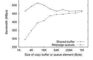
Figure 2: Bandwidth of three memory copy implementations
