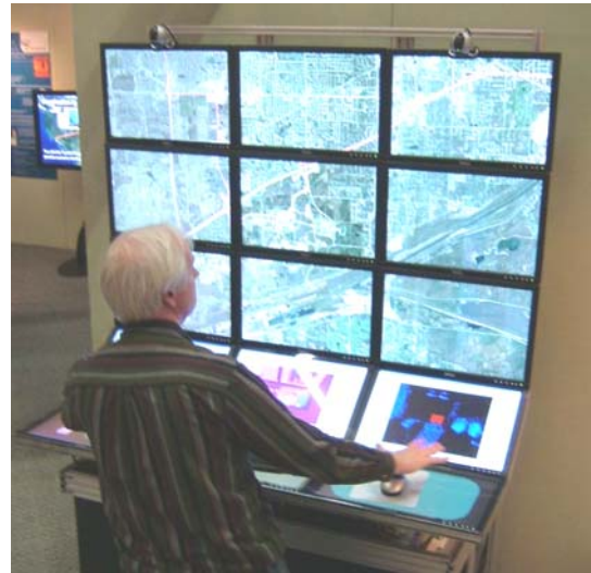
Figure 3: The CupHolder. The angled console and horizontal table surfaces both provide substantial pixel real estate for application control interfaces that may involve gesture recognition.
