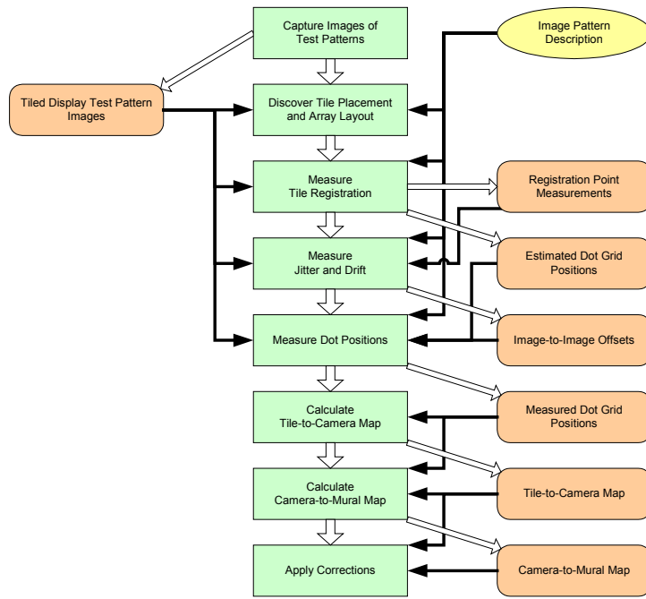
Figure 1 Schematic of the processing steps. The steps in the process are shown in the middle column and are represented by rectangles. Input to the process in the form of a geometrical description of the test pattern (see Figure 2) is shown as an oval. Rounded rectangles in the left and right columns are data products created and consumed in the process. Wide white arrows indicate process flow. Thinner white arrows indicate data creation. And, narrow black arrows indicate data consumption.
