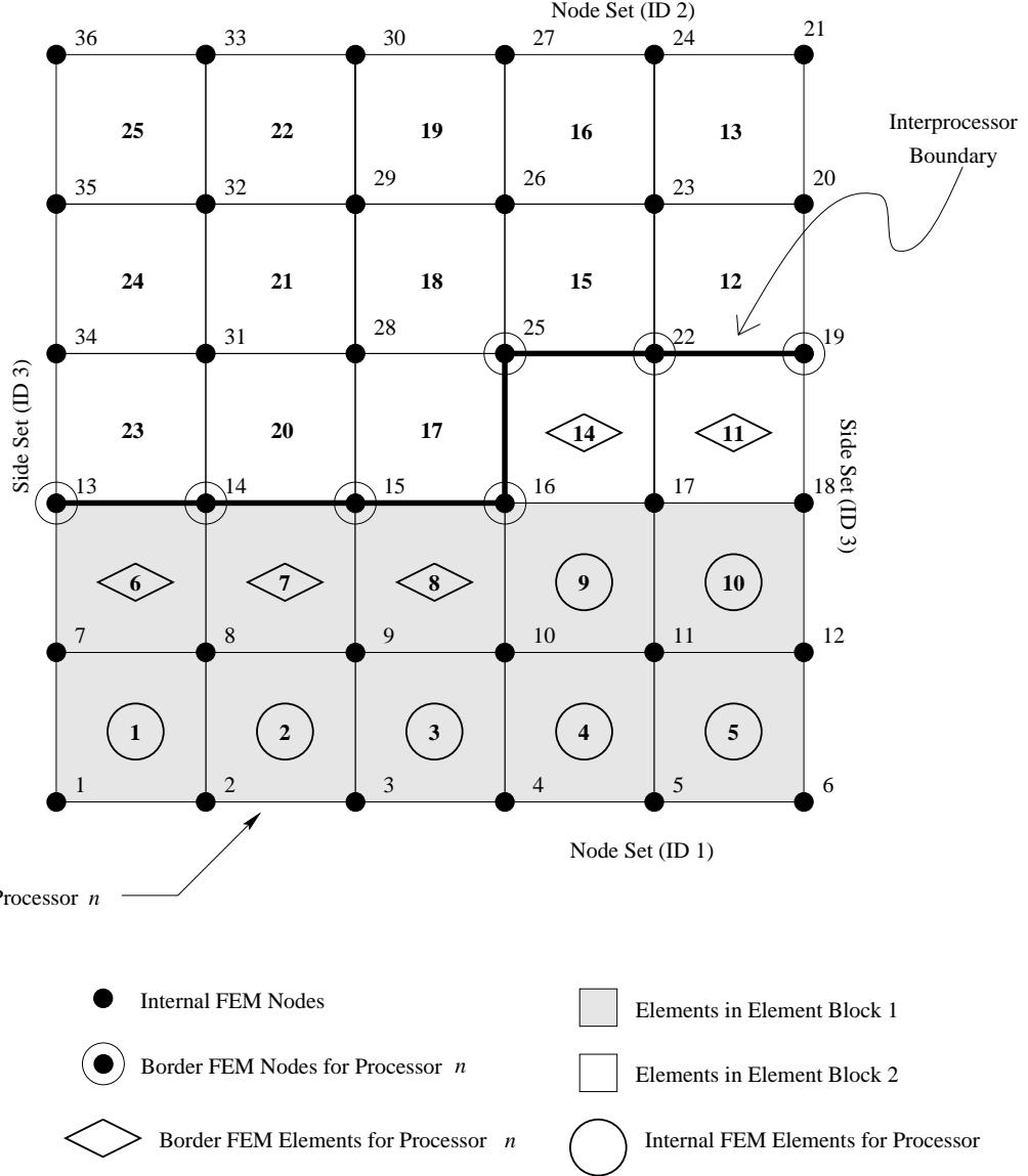
Figure 5: Elemental based decomposition example geometry.
